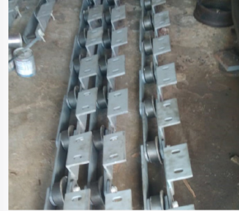
FABRICATION OF APRON WHEEL & APRON LINK PT PLN Indonesia Power UBP Suralaya Unit 1-7
