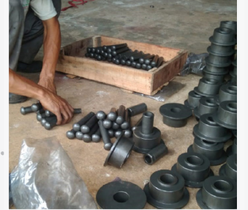
FABRICATION OF APRON WHEEL & APRON LINK PT PLN Indonesia Power UBP Suralaya Unit 1-7
