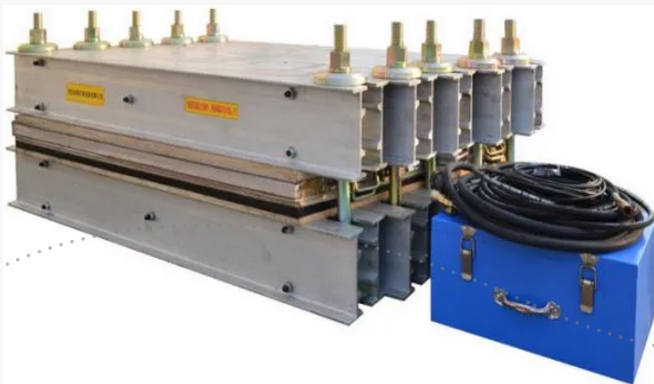
OUR BELT SPLICING/VULCANIZING MACHINE
