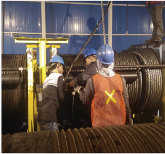
SHIP UNLOADER SLING WIRE ROPE REPLACEMENT SERVICES PT Lestari Banten Energi
